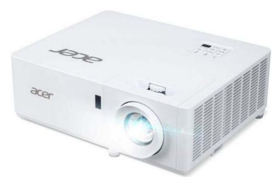
The Acer model VL6530i is a DLP laser projector with HDTV 1920 x 1080 resolution and a contrast of 2000000:1. The service life is 20000 hours due to the laser, which is the equivalent of over 13.7 years at 4 hours. With the lens shift function, the projector can be positioned very freely. An image width of up to 643 cm is possible, if the image width is smaller (we recommend
